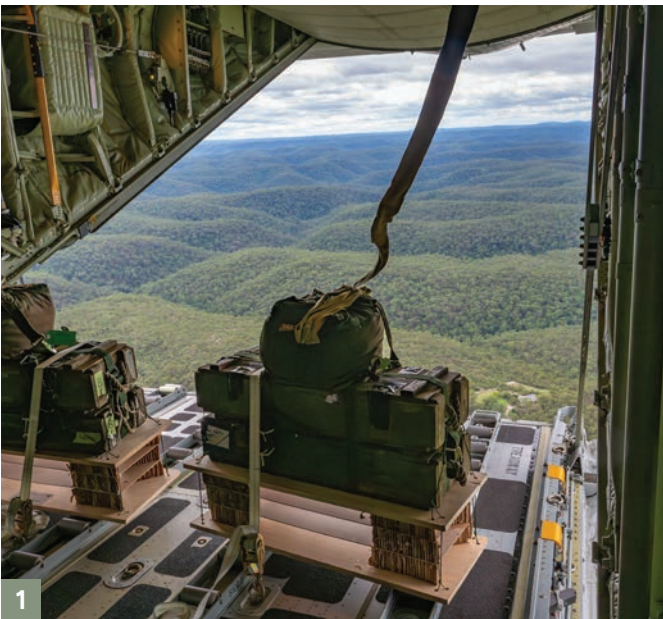
Compact loads restrained on the ramp of a U.S. C-130 Hercules aircraft prior to being dispatched to the drop zone during an interoperability activity. Photographer: CPL Shannon Gordon
