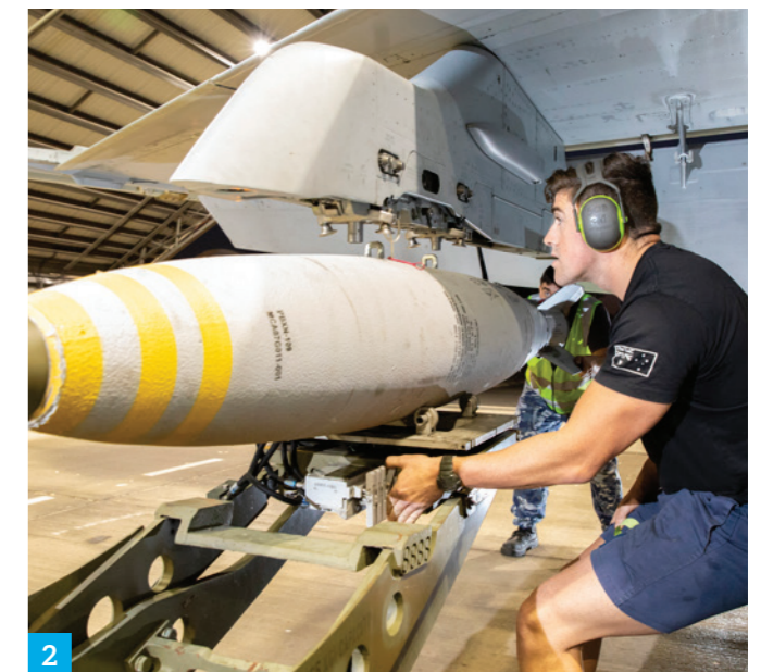
2 Royal Australian Air Force Armament Technicians Corporal Damien Powers (L) and Leading Aircraftman Joshua Sciberras (R) from No. 75 Squadron load a Mark 83 AIR high explosive ordnance onto a F/A-18A Hornet during Exercise Arnhem Thunder 21.
